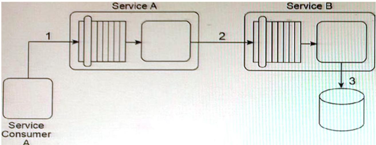
The data model used by Service Consumer A to represent the invoice document is based on XML Schema A. The service contract of Service A is designed to accept invoice documents based on XML Schema
