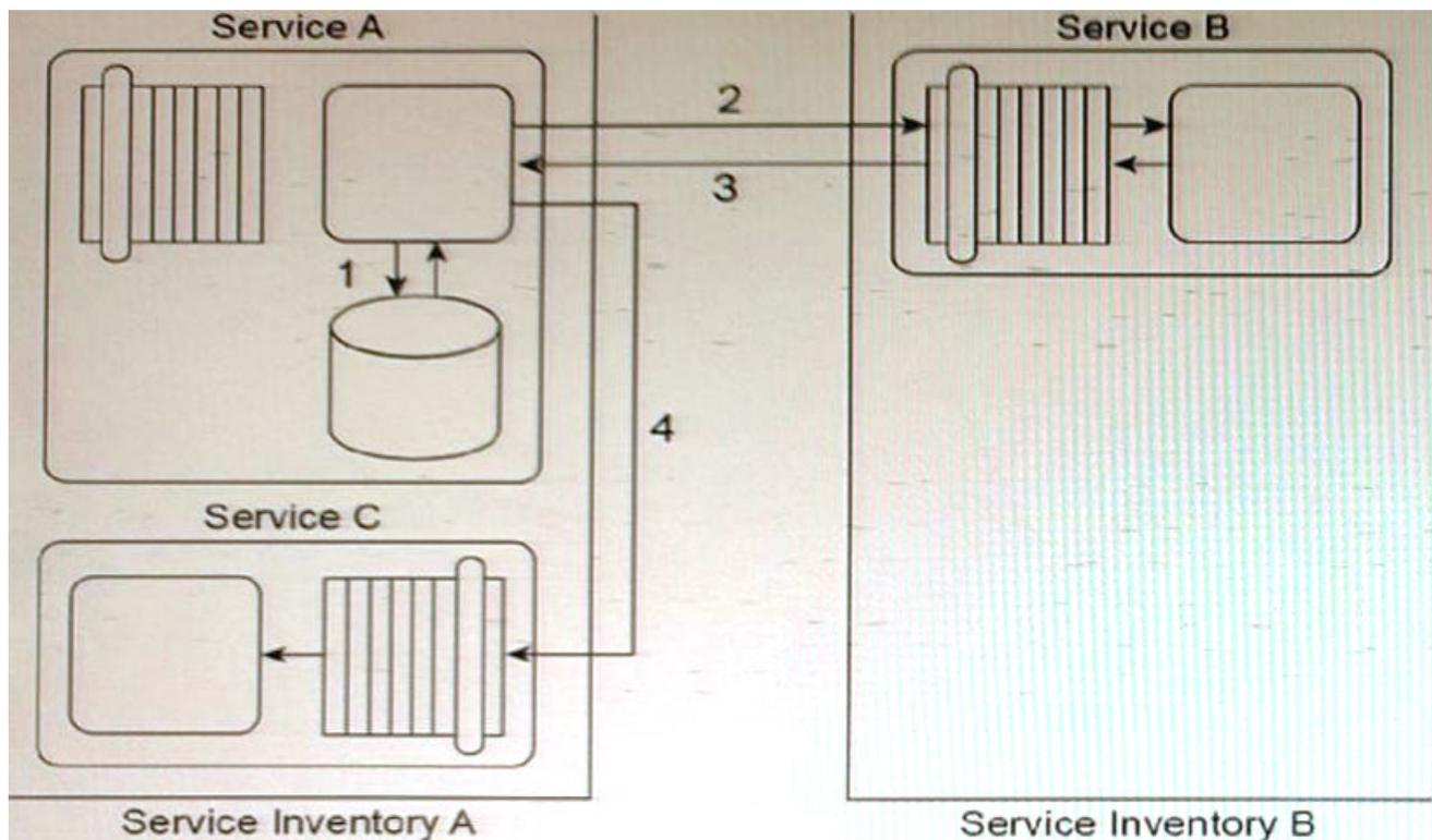
Before it contacts Service B, Service A must first retrieve a list of code values from its own database (1) and then place this data into its own memory. If it turns out that it must send a message to Service C, then Service A must combine the data it receives from Service B with the data from the code value list in order to create the message it sends to Service C. If Service A is not required to invoke Service C, it can complete its task by discarding the code values.
