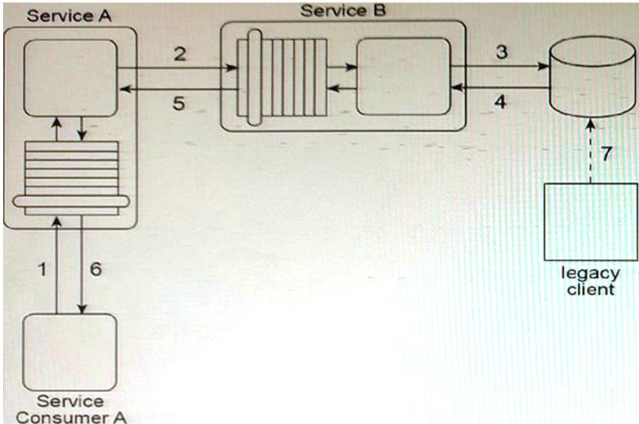
Service Consumer A invokes Service A in order to request this data value (1). For Service A to carry out this request, it must invoke Service B (2), a utility service that interacts (3, 4) with the database in which the data value is stored. Regardless of whether the data value changed, Service B returns the latest value to Service A (5), and Service A returns the latest value to Service Consumer A (6).
