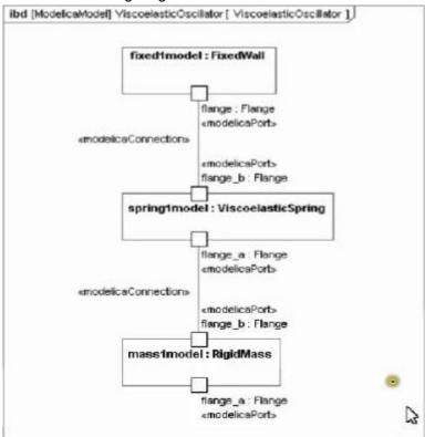
Assume that all stereotypes required by the SysML-Modehca Transformation specification (if any) have been applied but are not necessarily shown here Assume that FixedWall. ViscoelasticSpring. and RigidMass are fully defined in a Modelica library.
