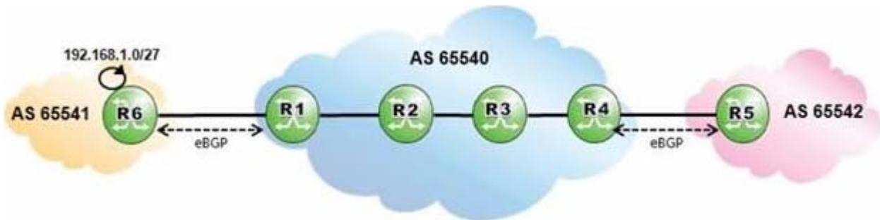
AS 65540 is using MPLS to provide BGP shortcuts for its iBGP routing.
