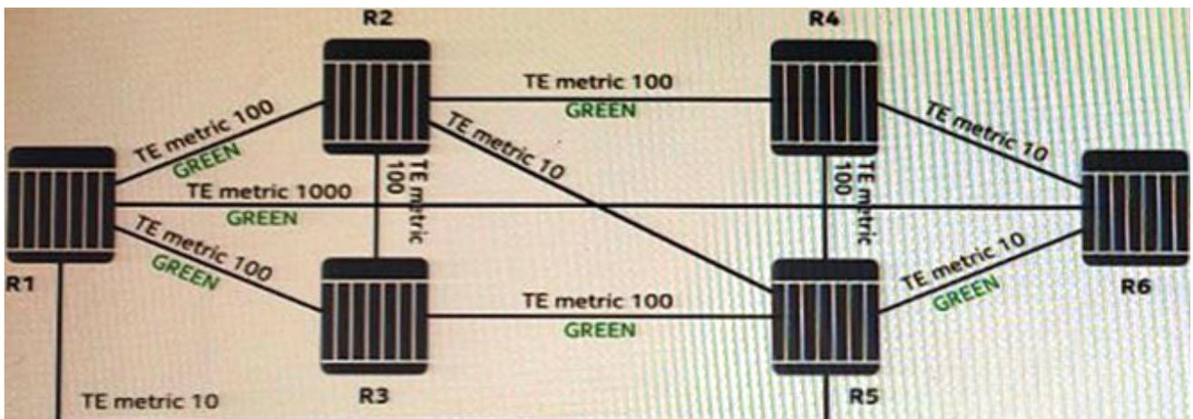
An LSP is being configured to start at R1 and end at R6 using local CSPF. The LSP has the following constraints. Include admin-group GREEN, use the TE metric and hop-limit 3.
