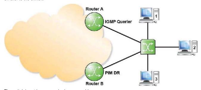
The switch is not igmp-snooping/proxy capable.
