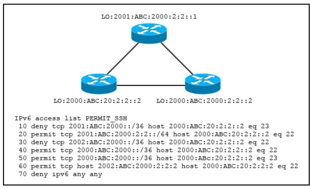
Which sequence number must be moved to the top pf the ACL to enable access from R3 to R2?
